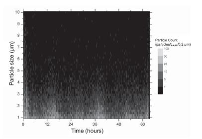
a) Time-resolved size histogram of total airborne particles in office room air
