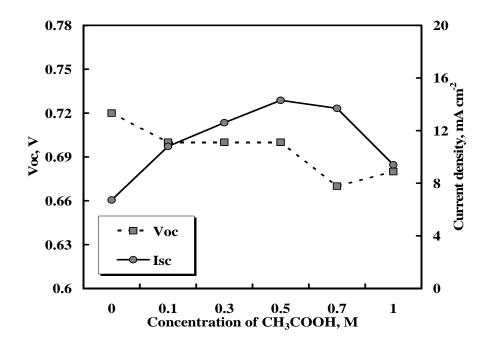
**FIG. 4** Current density with the concentration of CH<sub>3</sub>COOH (a) open circuit voltage is square symbol, (b) short circuit current is circle symbol
