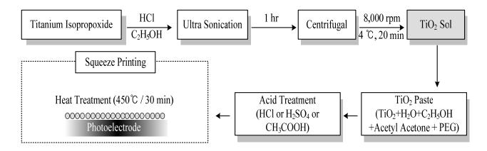
FIG. 1 Flow chart of TiO2 sol synthesis and photoelectrode fabrication process
