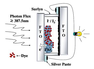
**FIG. 2** The device structure of dye sensitized solar cell which is consisted with the photoelectrode, organic dye, electrolyte containing with redox couple and counter electrode.
