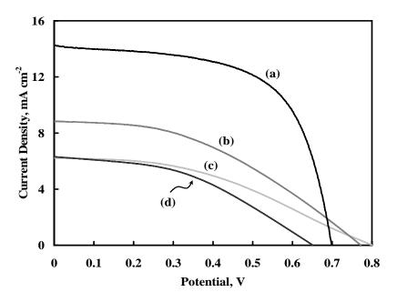
FIG. 3 Photocurrent-photovoltaic (J–V) characteristics of acid treated TiO<sub>2</sub> nano particles of DSSCs (a) CH<sub>3</sub>COOH, (b) HCl (c) None acid and (d) H<sub>2</sub>SO<sub>4</sub>
