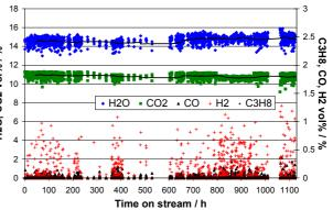
Fig.1b: 1,000 hours stability test for self-developed catalyst for total oxidation of propane (750°C)
