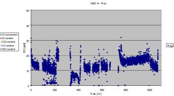
Fig.1c: 1,000 hours stability test for self-developed catalyst for water-gas shift
