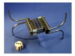
Fig. 6 Reactor/heat-exchanger for the preferential oxidation of carbon monoxide
