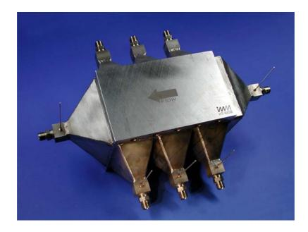
Fig.4: 5 kW high temperature water-gas shift reactor with cross-flow cooling capabilities
