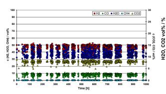
Fig.1a: 1,000 hours stability test for self-developed catalyst for propane steam reforming
