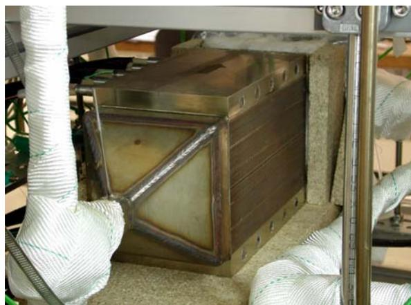
Fig.4: LT-WGS reactor
