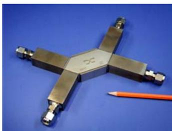
Fig.6 2 kW heat-exchanger applied for cooling the reformat
