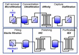
Fig.1: Typical downstream process for biological products
