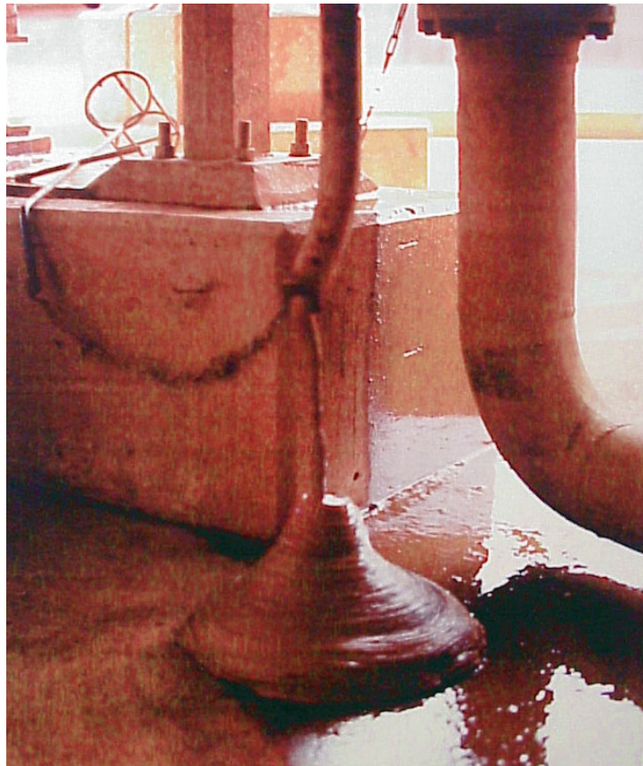
Figure 2: Mineral waste produced with a compression thickener.
