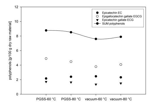
Figure 2: Plot showing polyphenol content in extracts dried with vacuum and PGSS (60  $^{\circ}$ C and 80  $^{\circ}$ C indicate temperatures at which extractions were performed)
