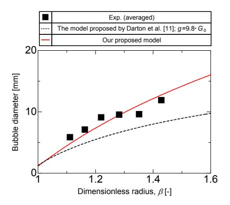
**Figure 5.** Bubble diameter as a function of dimensionless radius.  $G_0=10.0$ ;  $(u-u_{mf})_{L=0}=0.170$  m/s.
