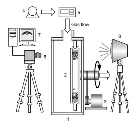
**Figure 3.** Experimental set up. (1) Plenum chamber; (2) rotating vessel (gas distributor; I.D. 250 mm  $\times$  D. 5 mm); (3) motor; (4) blower; (5) mass flow meter; (6) high-speed video camera; (7) data acquisition system for high-speed video camera; (8) metal halide lamp.
