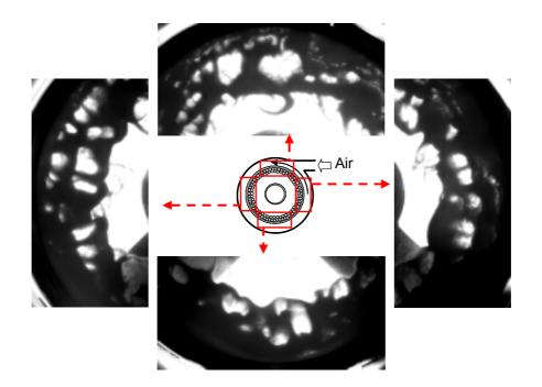
**Figure 4.** Visualized bubbling behavior in RFB.  $G_0=20.0$ ;  $(u-u_{mf})|_{L=0}=0.170$  m/s.
