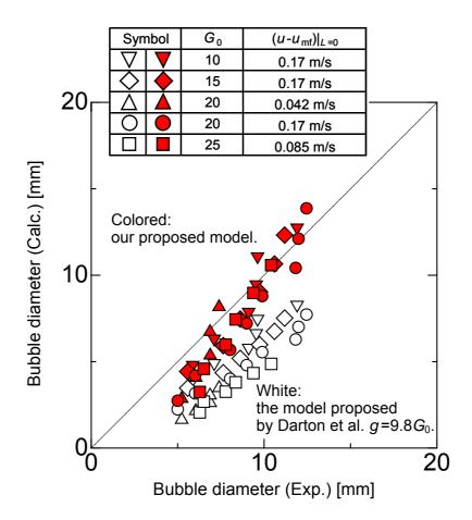
**Figure 6.** Comparison between experimental and estimated results of bubble diameters. Colored and white symbols indicate the estimated results by our proposed model and the model proposed by Darton et al. [11], respectively.
