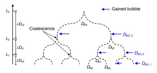
Figure 2. Schematic diagram of the proposed bubble growth model in RFB.
