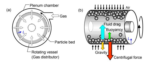
Figure 1. Rotating fluidized bed (RFB) system. (a) Front view; (b) side view.
