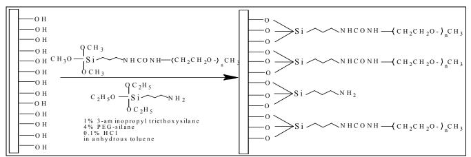
Figure 2: Schematic of surface modification of microchip by a mixed self assembled-monolayer of PEG-silane and aminosilane. The resultant free amino terminals are used for attachment of amino acids to build up cell adhesive peptide sequences.
