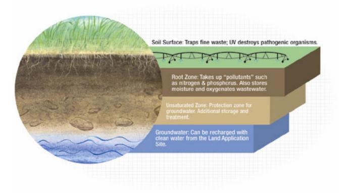
Figure 1. Land Application System Profile (courtesy Cascade Earth Sciences)
