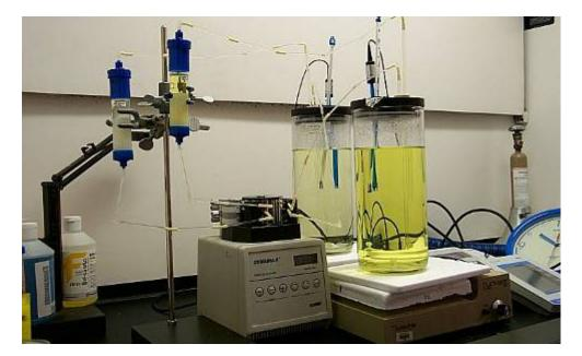
**Figure 8.** OPAA-Agarose (front) and BSA-Agarose (rear) 2 liter systems after the five day treatment of paraoxon in tap water. The yellow compound is the *p*-nitrophenolate ion of *p*-nitrophenol, one of the paraoxon hydrolysis products.
