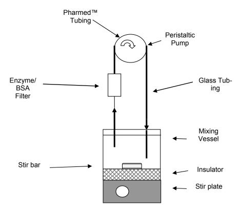
Figure 4. Reverse circulating filter loop system used in the 50 and 2000 ml systems.
