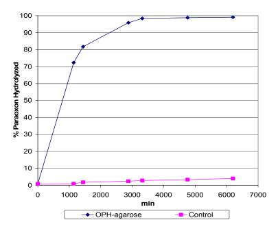
**Figure 5.** 5 day paraoxon catalysis by OPH-agarose in the 50 ml reverse circulating enzyme filter loop system.
