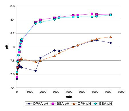
**Figure 9.** pH profile of the catalytic and control filter loops during paraoxon hydrolysis in the 2 liter systems.
