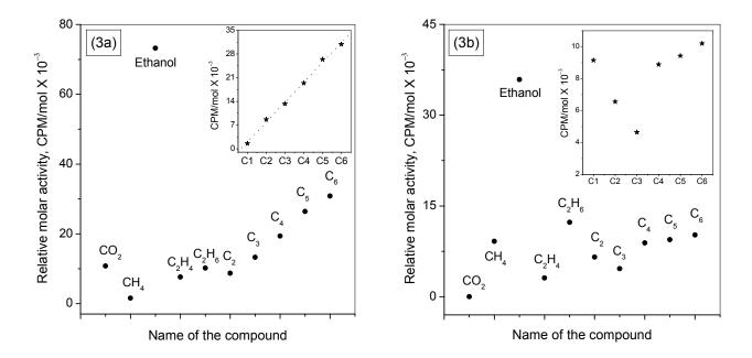
**Figure 3.** The relative molar <sup>14</sup>C activity of gaseous products after addition of labeled acetic acid during FTS at 270 °C, 100 psig,  $H_2/CO = 1.2$  with a doubly promoted iron catalyst (CO conversion ca. 85%): (a) 1-<sup>14</sup>C labeled acetic acid at a flow rate of 1.51 mL/h for 7 h; (b) 2-<sup>14</sup>C labeled acetic acid at a flow rate of 1.49 mL/h for 7.5 h.
