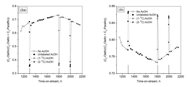
**Figure 2.** Variation of olefin/hydrocarbon ratio against reaction time during addition of labeled and unlabeled acetic acid in FTS at 270 °C and 100 psig: (a)  $C_2$  olefin/ $C_2$  hydrocarbons; (b)  $C_3$  olefin/ $C_3$  hydrocarbons. The dotted line on the TOS axis indicates the starting time for acetic acid addition while the solid line indicates the time when the addition was stopped.
