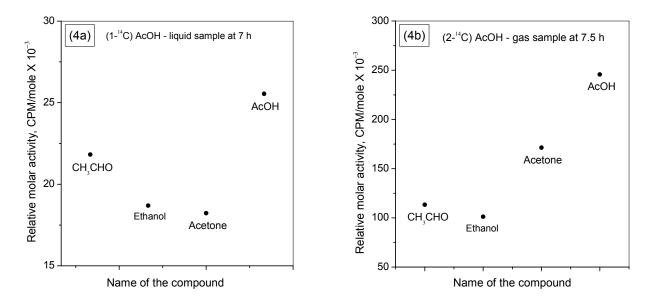
**Figure 4.** The relative molar <sup>14</sup>C activity of oxygenates (in the aqueous phase) after addition of labeled acetic acid during FTS at 270 °C, 100 psig,  $H_2/CO = 1.2$  with a doubly promoted iron catalyst (CO conversion ca. 85%): (a) 1-<sup>14</sup>C labeled acetic acid at a flow rate of 1.51 mL/h for 7 h; (b) 2-<sup>14</sup>C labeled acetic acid at a flow rate of 1.49 mL/h for 7.5 h.
