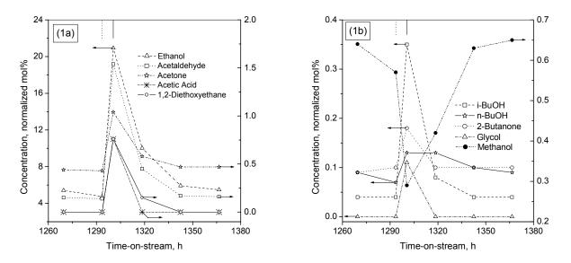
**Figure 1.** Variation in the concentration (in aqueous phase) of different oxygenates produced in FTS at 270 °C and 100 psig with addition of unlabelled acetic acid (flow rate of 1.43 mL/h for 7 h). The dotted line on the TOS axis indicates the starting time for acetic acid addition while the solid line indicates the time when the addition was stopped.
