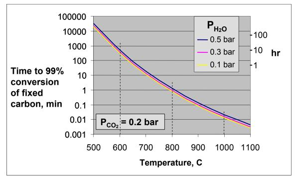
In this paper, we examine the impact of process conditions – temperature, pressure, and gasifying agent on carbon gasification kinetics and conversion, tar production, and sulfur speciation. The results presented are discussed in terms of gasifier design, gas clean-up and conditioning requirements, and energy recovery as products.
