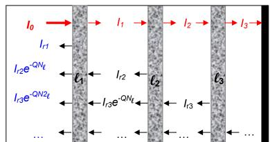
Figure 1 - Model of Reflected Light Intensity Measurement
