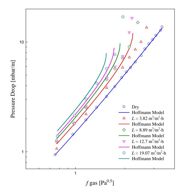
**Figure 2.** Pressure drop behavior for KATAPAK-SP 12. Calculations using original model parameters. Experimental points from Ratheesh and Kannan<sup>2</sup>
