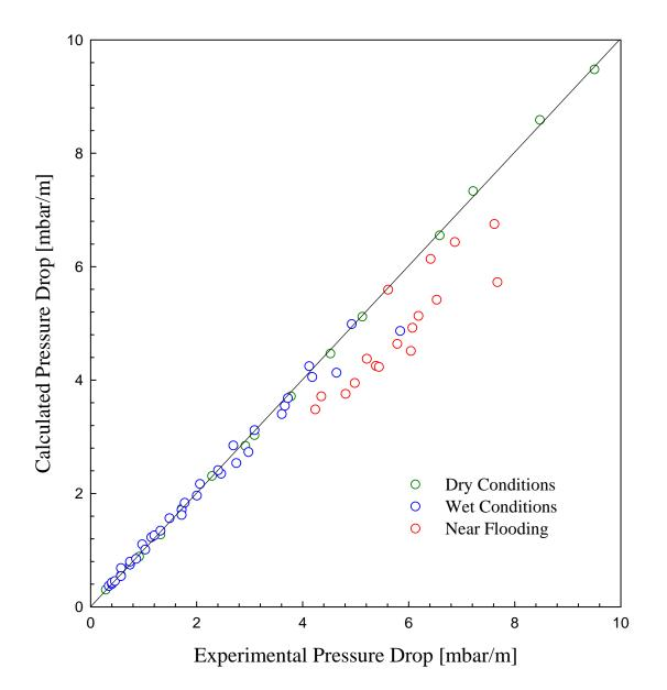
**Figure 1.** Calculated pressure drop for KATAPAK-SP 11 vs. experimental values. Calculations using original model parameters. Experimental data from Brunazzi et al.<sup>3</sup>
