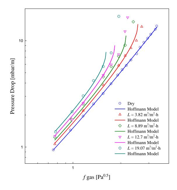
**Figure 4.** Pressure drop behavior for KATAPAK-SP 12. Calculations using modified Hoffmann model. Experimental points from Ratheesh and Kannan<sup>2</sup>
