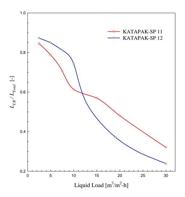
Figure 5. Variation of  $L_{CB}/L_{total}$  with liquid load for the two CSP under study
