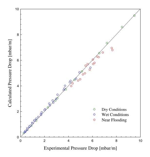
**Figure 3.** Calculated pressure drop for KATAPAK-SP 11 vs. experimental values. Calculations using modified Hoffmann model. Experimental data from Brunazzi et al.<sup>3</sup>
