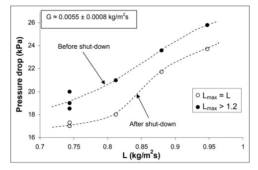
Figure 2. Experimental hysteresis behaviour at different liquid flow rates
