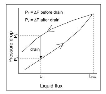
Figure 3. Qualitative hysteresis behaviour with liquid flow (after Levec et al., 1986)
