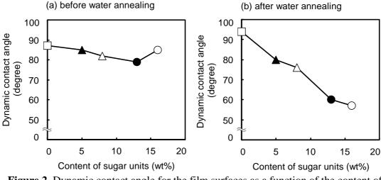
**Figure 2.** Dynamic contact angle for the film surfaces as a function of the content of sugar units. (a) Before annealing in water, (b) After annealing in water.<sup>5</sup>
