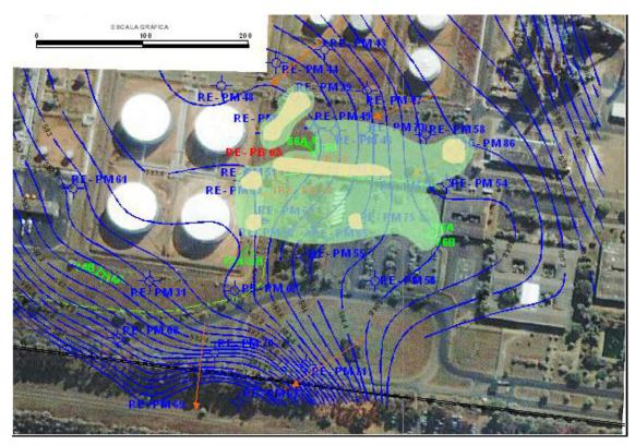
Figure 1: Free-phase jet fuel area (July- 2006)
