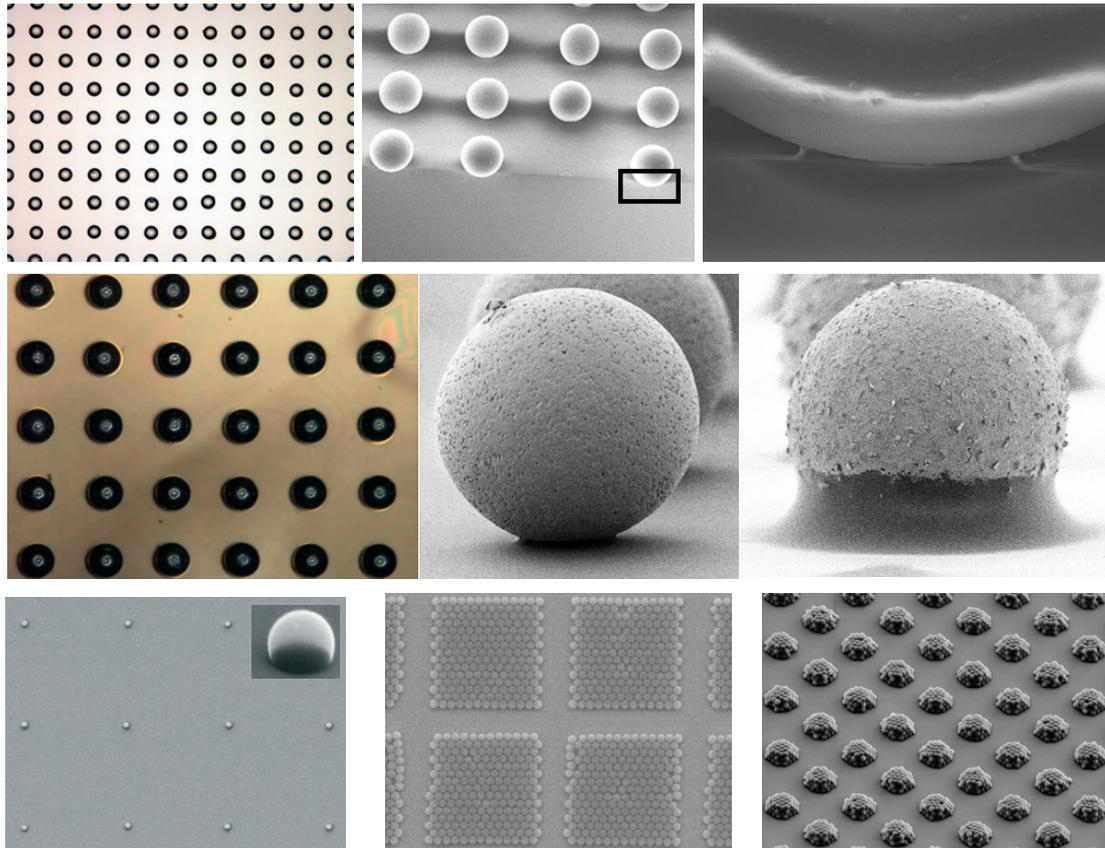
Figure 3: Arrays of 100- $\mu\text{m}$  glass beads (top row), 100- $\mu\text{m}$  tin-coated beads (second row) and 500-nm polystyrene particles (third row), assembled and printed using the SATI process.
