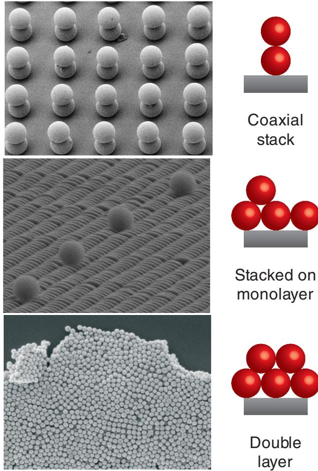
Figure 4: Stacks of 100- $\mu\text{m}$  glass, 500-nm polystyrene and 60-nm gold particles (from top to bottom).
