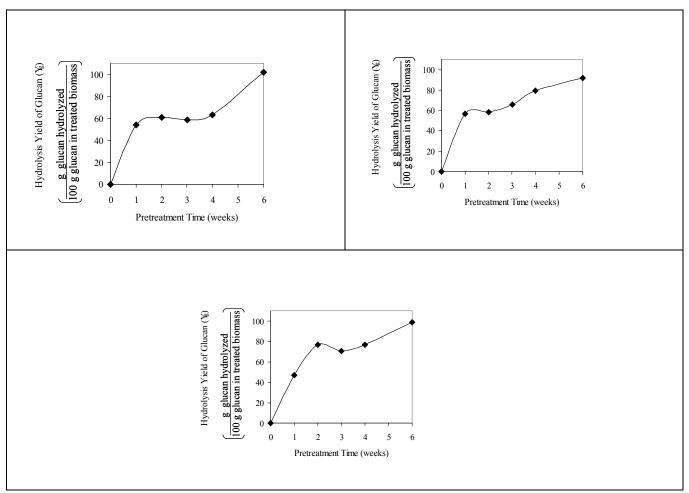
**Figure 5**. Enzymatic hydrolysis yield of glucan for poplar wood (LLB) pretreated at the following conditions: a) 55°C b) 65°C and c) 75°C
