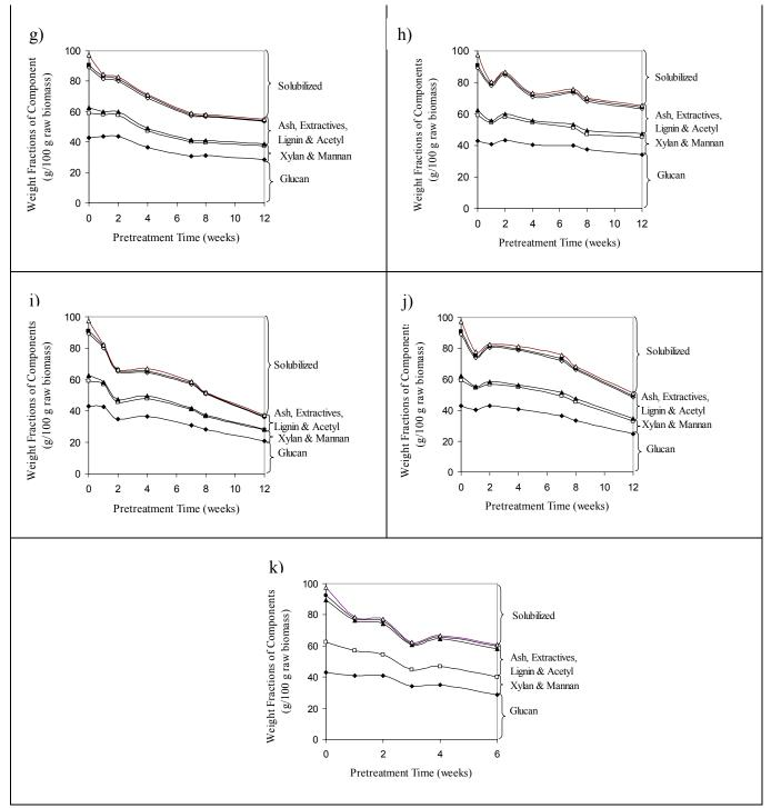
**Figure 2.** (*Continued*). Mass balances after pretreatment for the High-Lignin Batch at the following conditions: g) 55°C and oxidative, h) 55°C and non-oxidative, i) 65°C and oxidative, j) 65°C and non-oxidative, k) 75°C and oxidative.
