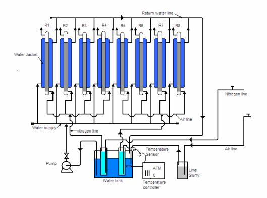
Figure 1. Diagram of a set of eight reactors in the reactor system for lime pretreatment.
