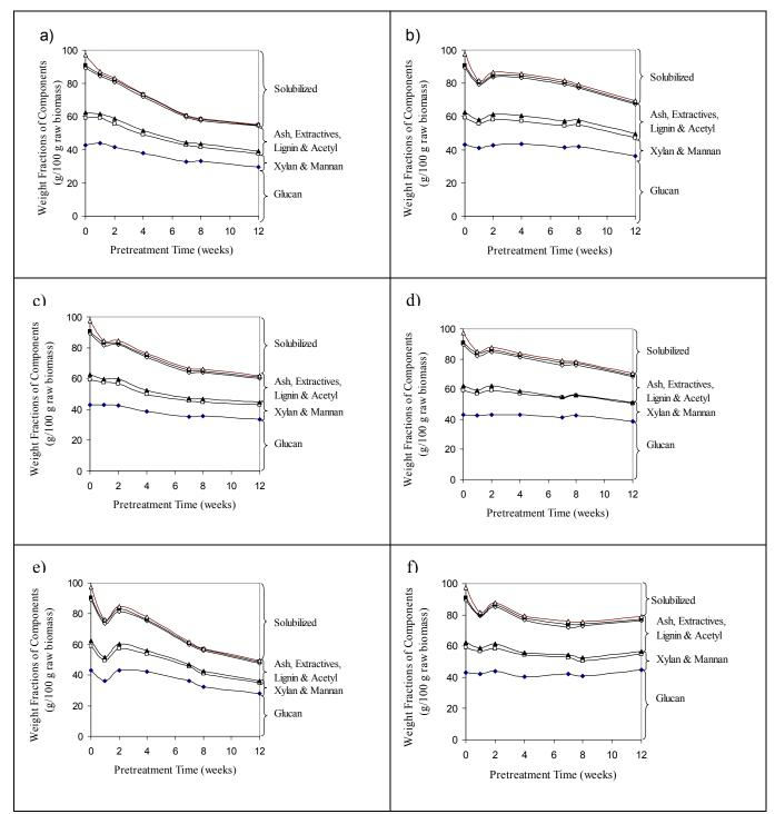
**Figure 2**. Mass balances after pretreatment for the High-Lignin Batch at the following conditions: a) 25°C and oxidative, b) 25°C and non-oxidative, c) 35°C and oxidative, d) 35°C and non-oxidative, e) 45°C and oxidative, g) 45°C and non-oxidative.
