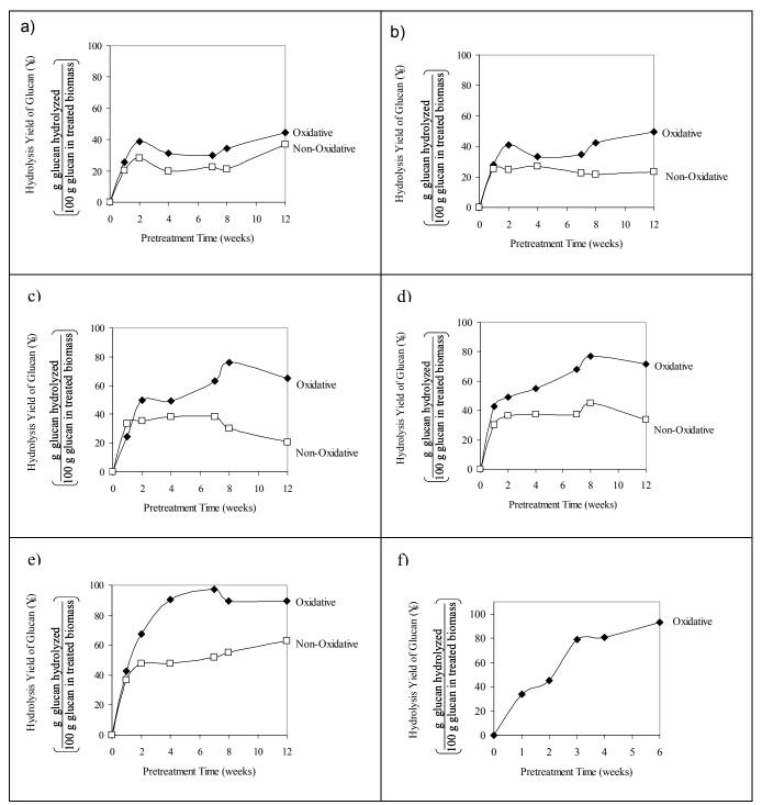
**Figure 4**. Enzymatic hydrolysis yield of glucan for poplar wood (HLB) pretreated at the following conditions: a) 25°C b) 35°C c) 45°C d) 55°C e) 65°C f) 75°C
