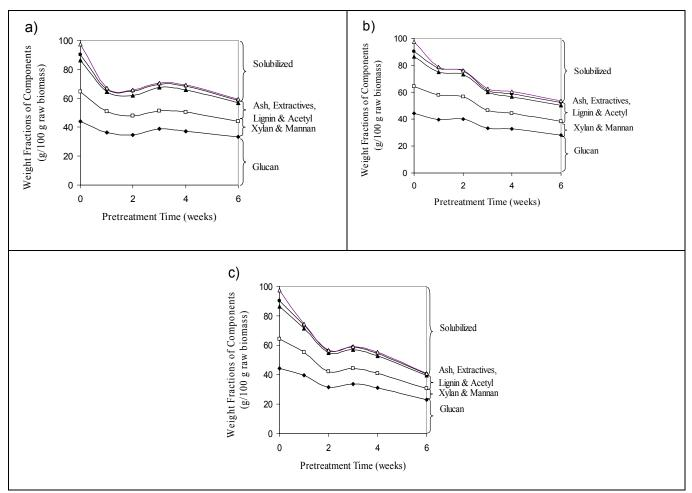
**Figure 3.** Mass balances after pretreatment for the Low-Lignin Batch at the following conditions: g) 55°C and oxidative, a) 55°C and non-oxidative, b) 65°C and non-oxidative, c) 75°C and oxidative.
