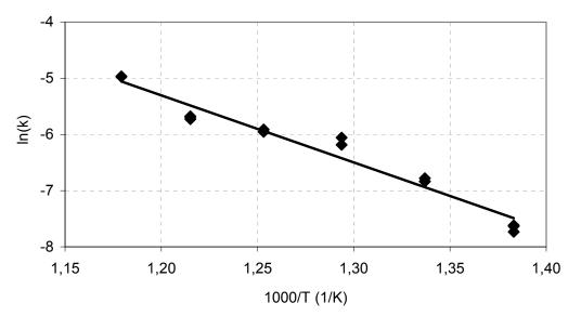
Figure 1: Arrhenius plot with an assumed first order rate constant for the 2CP hydrolysis in acid media at 280 bar from 450 to 575°C
