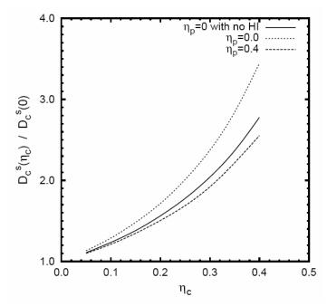
Fig.3: Short-time (macroscopic) collective diffusion coefficient of colloids in solution with and without polymer. The case where hydrodynamic interactions (HI) are absent is also plotted for reference.  $\beta = a/R = 0.216$  and q = 0.4.
