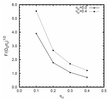
Fig.4: Long-time mobility factor of colloids in solutions with and without polymer.  $\beta = a/R = 0.216$  and q = 0.4.
