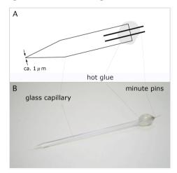
Fig. 1 Structure of micropump
