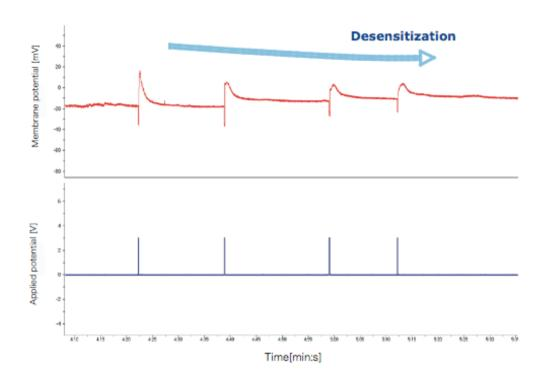
**Fig. 3:** Time course of membrane potential (upper) and applied potential toward electrode in the micropump filled with sodium glutamate solution.
