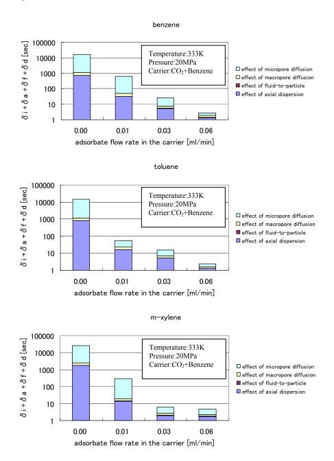
Figure.5 Contribution of four mass transfer steps
