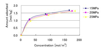
Figure.2 Adsorption isothem: benzene at 313K
