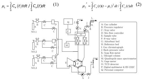
Figure I. Experimental apparatus
