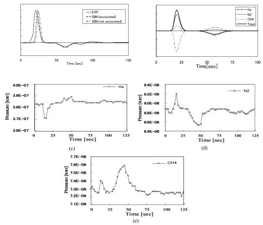
**Figure 6.** Comparison between experimental chromatogram and simulated one (a), Simulation of pulse response of each component (b), Experimental peak of Helium by mass detector (c), Experimental peak of  $N_2$  by mass detector (d) and Experimental peak of CH<sub>4</sub> by mass detector (e)
