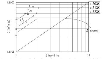
Figure 5. Correlation based on chemical potential driving force
