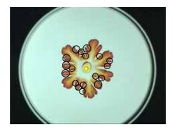
Figure 5. Reaction region in reactive miscible viscous fingering at t=150 s at  $\varphi_v=1$  ( $c_{l0}=0.04$  mol/l and  $c_{m0}=0.08$  mol/l) under the condition of b=0.3 mm and q=1.8 mm<sup>3</sup>/s. Blood red color region except the region specified by black circles indicates the reaction region, while the black circles represent the region in which the reaction does not take place although the product exists.
