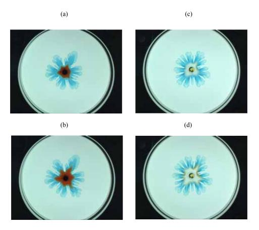
Figure 2. Viscous fingering pattern without and with the reaction when  $t_{sw}$ =90 s. (a) without reaction at t=120 s; (b) without reaction at t=150 s; (c) with reaction at t=150 s.
