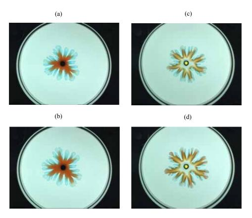
Figure 4. Viscous fingering pattern without and with the reaction when  $t_{sw}$  =30 s. (a) without reaction at t=120 s; (b) without reaction at t=150 s; (c) with reaction at t=150 s.
