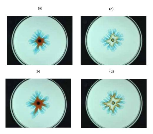
Figure 3. Viscous fingering pattern without and with the reaction when  $t_{sw}$ =60 s. (a) without reaction at t=120 s; (b) without reaction at t=150 s; (c) with reaction at t=150 s.
