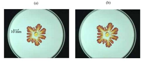
Figure 1. Reactive viscous fingering pattern when  $\varphi_v=1$  ( $c_{l0}=0.04$  mol/l and  $c_{m0}=0.08$  mol/l) under the condition of b=0.3 mm and q=1.8 mm<sup>3</sup>/s (a) at t=120 s and (b) at t=150 s.
