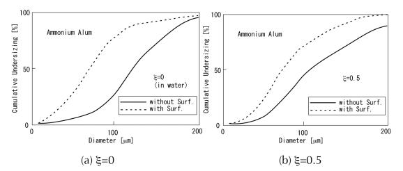
Figure 5 Cumulative Undersizing of Ammomium Alum Hydrates in Slurries
