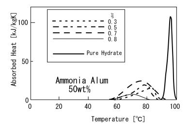
Figure 3 DSC Curves of Ammonium Alum Slurries
