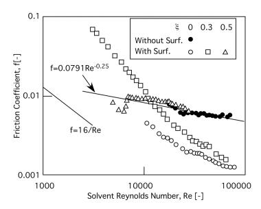
Figure 4 Friction Coefficient of the Mixture Treated with Surfactants
