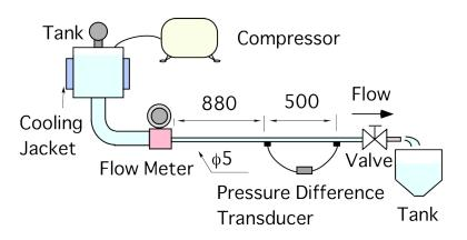
Figure 1 Once-through Flow System for Drag Reduction Effect
