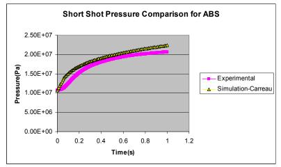
Fig.2. Pressure comparison for ABS short shot
