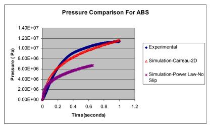
Fig.1. Pressure comparison for ABS full shot
