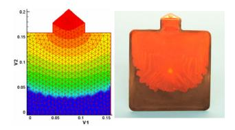
Fig.3. Fill pattern comparison for ABS full shot
