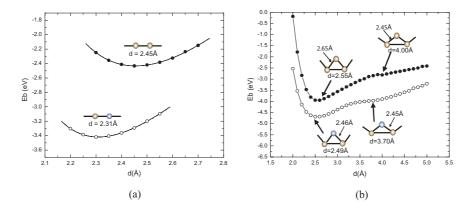
Figure 1: Calculated binding energy of Pd and Pd/Ni chain atoms per unit cell as function of length of unit cell d. Two geometries: (a) straight, (b) zigzag chains are shown as functions of d. The stable narrow angle and metastable wide angle zigzag chains are marked in the right figure. Black and white filled circles are for Pd and Pd/Ni chains, respectively. The binding energy is calculated from total energy difference between atomic chain and isolated atoms.
