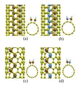
Figure 11: 3D views of equilibrium geometries of the  $H_2$  adsorbed Pd and Pd/Ni functionalized SWNTs. The color scheme is same as previous figures. Small bright blue dots are hydrogen atoms. (a) and (b) are SWNT(6,6) systems, (c) and (d) are SWNT(10,0) systems.
