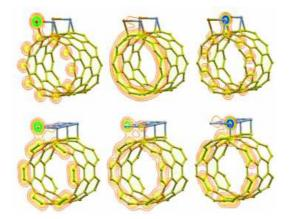
Figure 9: Contour plot of total (spin-up and spin-down) valence charge density on three planes for Pd/Ni chain functionalized SWNT(10,0) (upper) and Pd/Ni chain functionalized SWNT(6,6) (lower). The planes are through the cross section of the tube and different location on the Pd/Ni chain.
