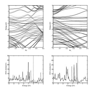
Figure 7: Spin-polarized band structure and DOS of (a) Pd/Ni narrow angle chain functionalized SWNT(6,6), and (b) Pd/Ni wide angle chain functionalized SWNT(10,0). Fermi level is set as zero.
