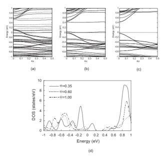
Figure 16: Spin-polarized band structure of hydrogen adsorbed on Pd radial chain-functionalized SWNT(10,0). From (a) to (c):  $\Theta$ =0.35, 0.60, 1.00. (d) Local DOS of Pd atoms at different  $\Theta$ .
