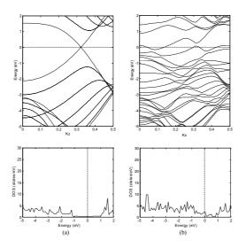
Figure 4: Spin-polarized band structure and DOS of (a) SWNT(6,6) and (b) Pd narrow angle chain adsorbed SWNT(6,6). Fermi level is set as zero.
