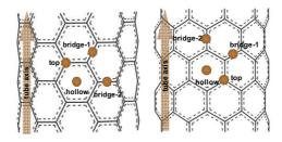
Figure 2: Schematic drawing of top views of four possible sites for single Pd atom adsorption on SWNT(6,6) and SWNT(10,0). Brown dots represent Pd atoms. Bridge-2 site differs from bridge-1 site in that the C-C bond is perpendicular to the tube axis at this site. In the SWNT(10,0) case, bridge-2 site is located on a C-C bond parallel to the tube axis.
