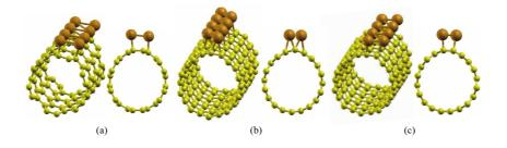
Figure 3: 3D view of equilibrium geometries of the Pd chain SWNT structures. (a) Pd narrow angle chain on top site of SWNT(6,6), (b) Pd wide angle chain on bridge-1 site of SWNT(10,0), (c) Pd wide angle chain on bridge-2 sites of SWNT(10,0). In all cases, changes in the tube shape are seen from the cross sectional views.
