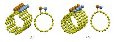
Figure 6: 3D views of equilibrium geometries of the Pd/Ni chain-tube structures. (a) Pd/Ni narrow angle chain on top site of SWNT(6,6), (b) Pd/Ni wide angle chain on bridge-2 site of SWNT(10,0).
