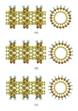
Figure 15: 3D views of equilibrium geometries of hydrogen adsorbed Pd radial chain-functionalized SWNT(10,0). From top to bottom:  $\Theta = 0.35$ , 0.60, 1.00.
