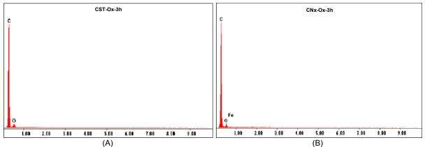
Figure 2. (A) Quantitative analysis of the CST modified for 3 h; (B) Quantitative analysis of the CNx modified for 3 h
