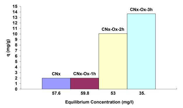
Figure 4. Cadmium adsorption capacity of CNx. Initial concentration of 60 mg/L, pH 6, and  $25^{\circ}$  C.
