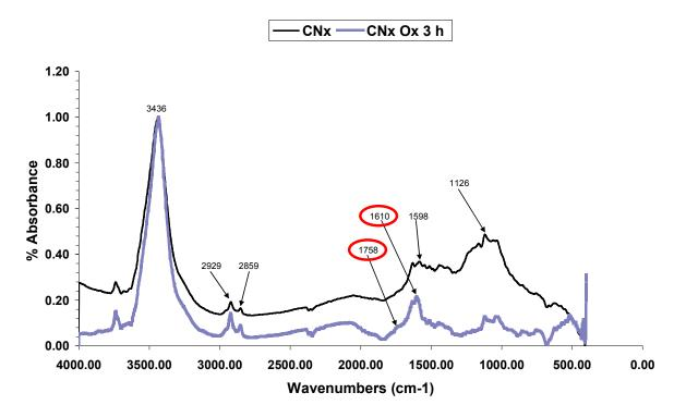
Figure 3. Infrared spectrum for CNx before and after its functionalization with HNO3
