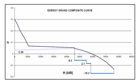
Fig 18: The refrigeration level placements on the Exergy Grand Composite Curve for existing refrigeration cycle
