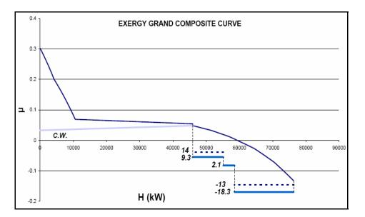
Fig 19: Exergy Grand Composite Curve with existing and proposal refrigeration levels
