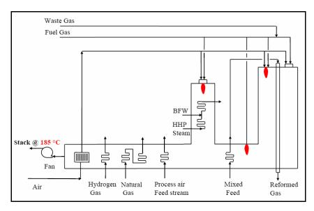
Fig. 10: The coil arrangement of the existing plant
