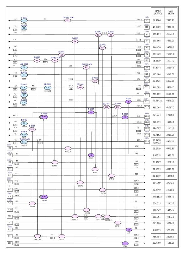
Fig. 12: Grid diagram of second retrofitted proposal
