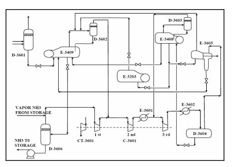
Fig 14: Schematic of ammonia refrigeration cycle
