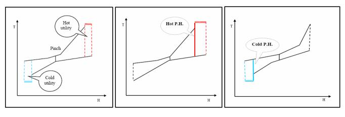
Fig.1: Composite curve
