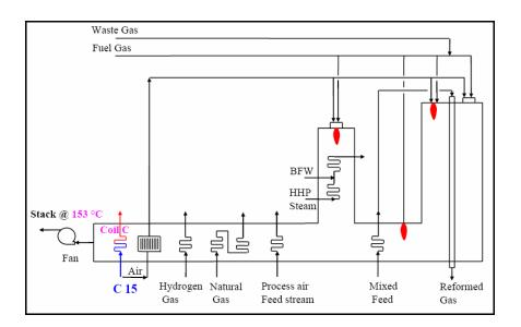
Fig. 11: The proposal coil arrangement
