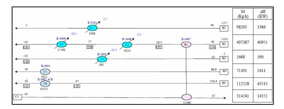
Fig. 15: Grid diagram of the existing HEN of cold section
