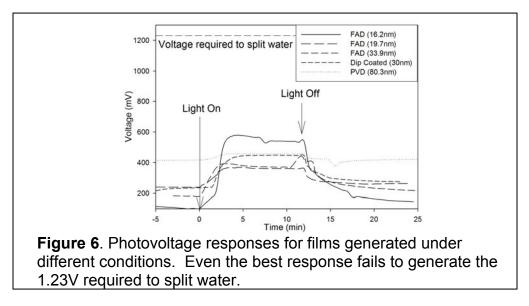
less than half of the required 1.23V required for the photosplitting of water. Again, films generated via  $FAD_3$  performed the best, with an increase in performance with decreasing primary particle size.
