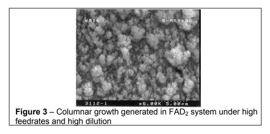
( $d_{pg}$ =73nm,  $\sigma_{g}$ =1.31). Particle density was high, and the primary direction of growth perpendicular to the surface (z direction). The resulting aggregates had the characteristic morphology of reaction-limited particle-cluster growth.<sup>13</sup>
