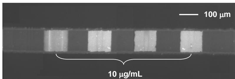
**Figure 7:** Performance assessment of the multi-target immunoassay. Concentration of coating *E. coli* lysate antigen was 10  $\mu\text{g}/\text{mL}$  for all sites.
