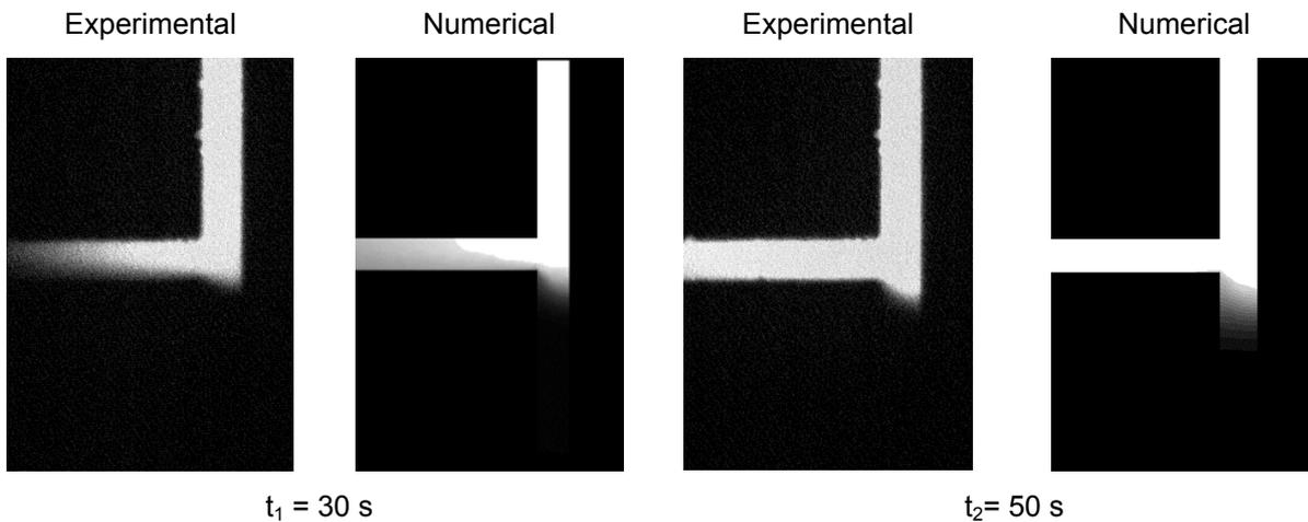
**Figure 6:** The second solution dispensing process (step 4) – experimentally and numerically acquired concentration fields on the right junction of the “H”.  $t_1$  and  $t_2$  indicate the lapse time after step 4 started.
