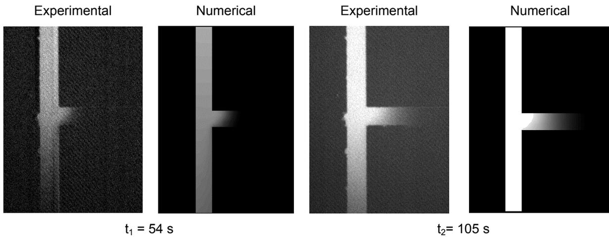
**Figure 5** The first solution dispensing process (step 1) – experimentally and numerically acquired concentration fields on the left junction of the “H”.  $t_1$  and  $t_2$  indicate the lapse time after step 1 started.
