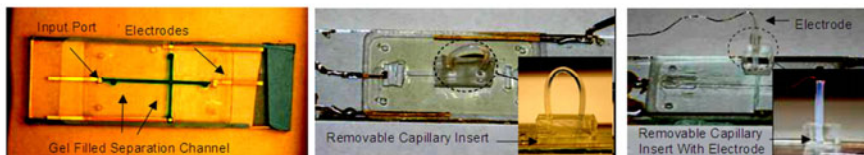
Figure 2 Images of micro 2D electrophoresis device fabricated using \mu Tectonics. (Left) Micro electrophoresis device before addition of RCI component. Channel is dyed green for imaging. (Center) Micro electrophoresis device with integrated RCI temporarily attached using a PDMS connector. (Right) Device with integrated RCI containing second electrode for electrophoresis. Once a protein or DNA is within the RCI, it is removed from the device for post separation analysis.
