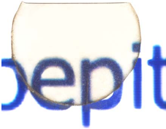
Fig. 6. Single crystal of (001) diamond grown by CVD on a Ir/SrTiO 3 substrate. The diameter is 3.5 mm; thickness is 35 μm. Note the absence of optical aberration and misoriented regions 24 .
