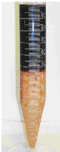
Figure 9 Gravity settling measurements of simulant over 1 hour
