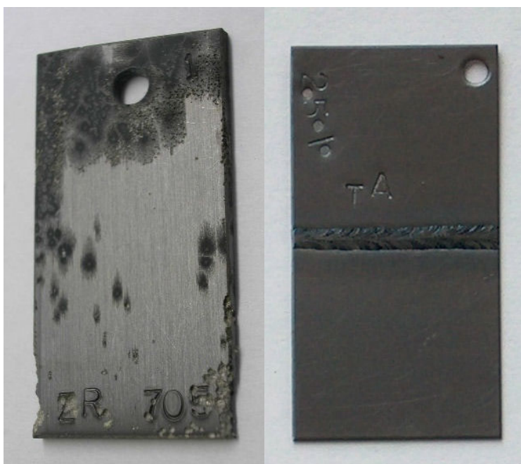
Figure 2: Zr-705 after 120 hours, Ta-2.5W after 1040 hours in \text{HI}_x . Zr-705 shows visible corrosion, while Ta-2.5W shows no corrosion.
