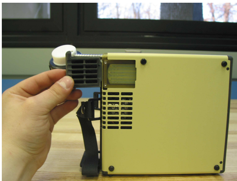
Figure 3 – SFC C20-MP air filtration system
