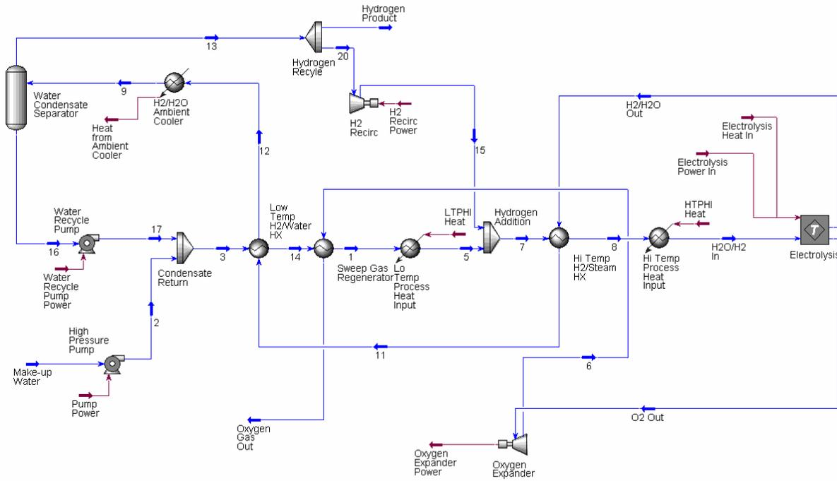
Figure 6. HYSYS process flow diagram for a 300 MW HTE plant with no sweep.
