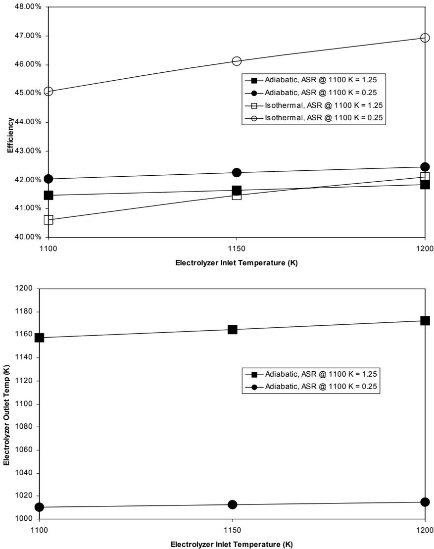
Figure 11. Overall thermal-to-hydrogen efficiencies (LHV) and electrolyzer outlet temperatures for Cases 17 – 20 (no sweep, fixed steam utilization, fixed current density of 0.25 A/cm<sup>2</sup>, 5 MPa).
