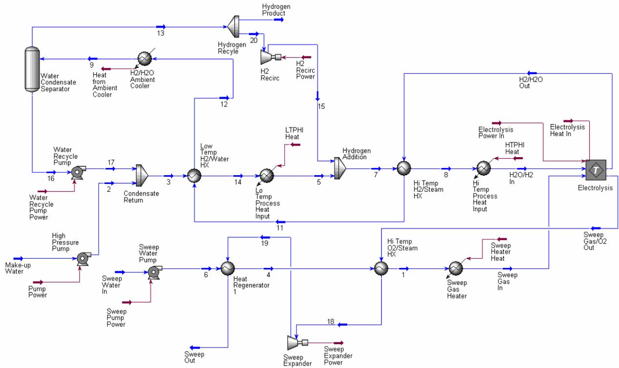
Figure 5. HYSYS process flow diagram for a 300 MW HTE plant with steam sweep.
