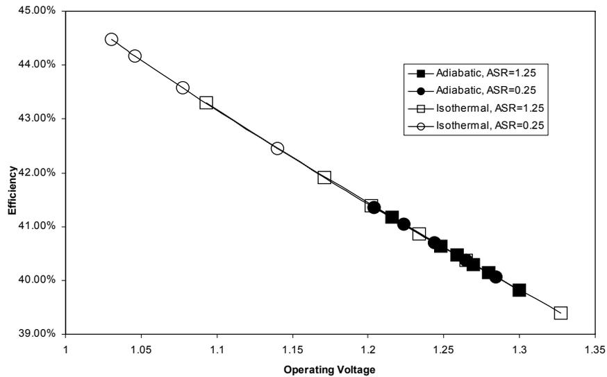
Figure 8. Overall thermal-to-hydrogen efficiencies (LHV) for Cases 5 – 8 (steam sweep, fixed steam utilization, 1100 K electrolyzer inlet temperature, 5 MPa).
