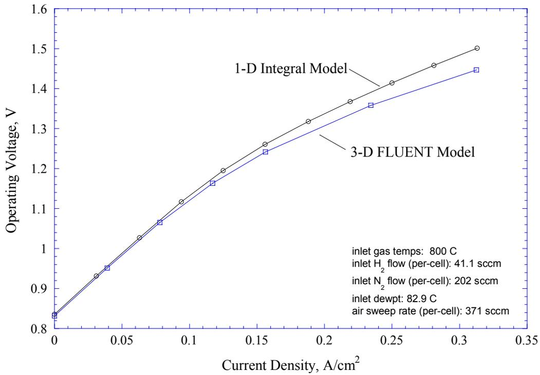
Figure 1. Operating voltage as a function of current density for adiabatic electrolyzer operation, predicted from a 1-D integral model and from a full 3-D FLUENT simulation.
