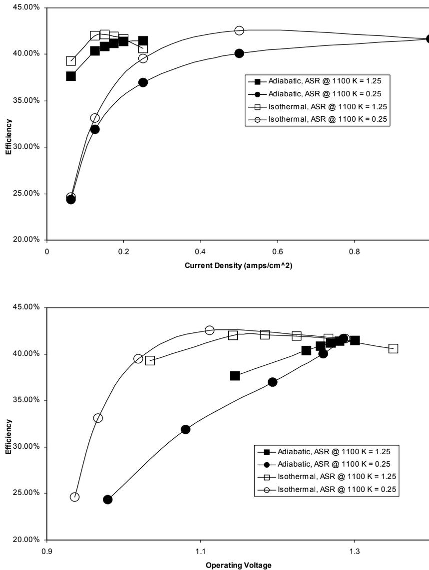
Figure 10. Overall thermal-to-hydrogen efficiencies (LHV) for Cases 13 – 16 (no sweep, fixed electrolyzer feed flowrate, 5 MPa).
