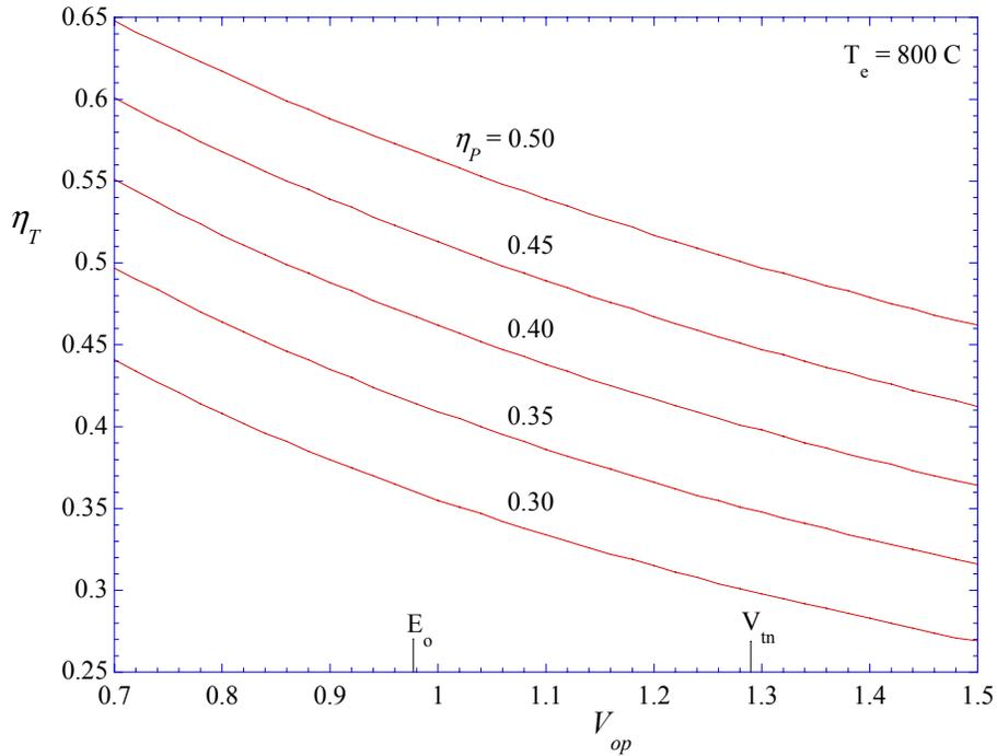
Figure 4. Electrolyzer overall hydrogen production efficiencies as a function of power-production thermal efficiency and electrolyzer per-cell operating voltage.
