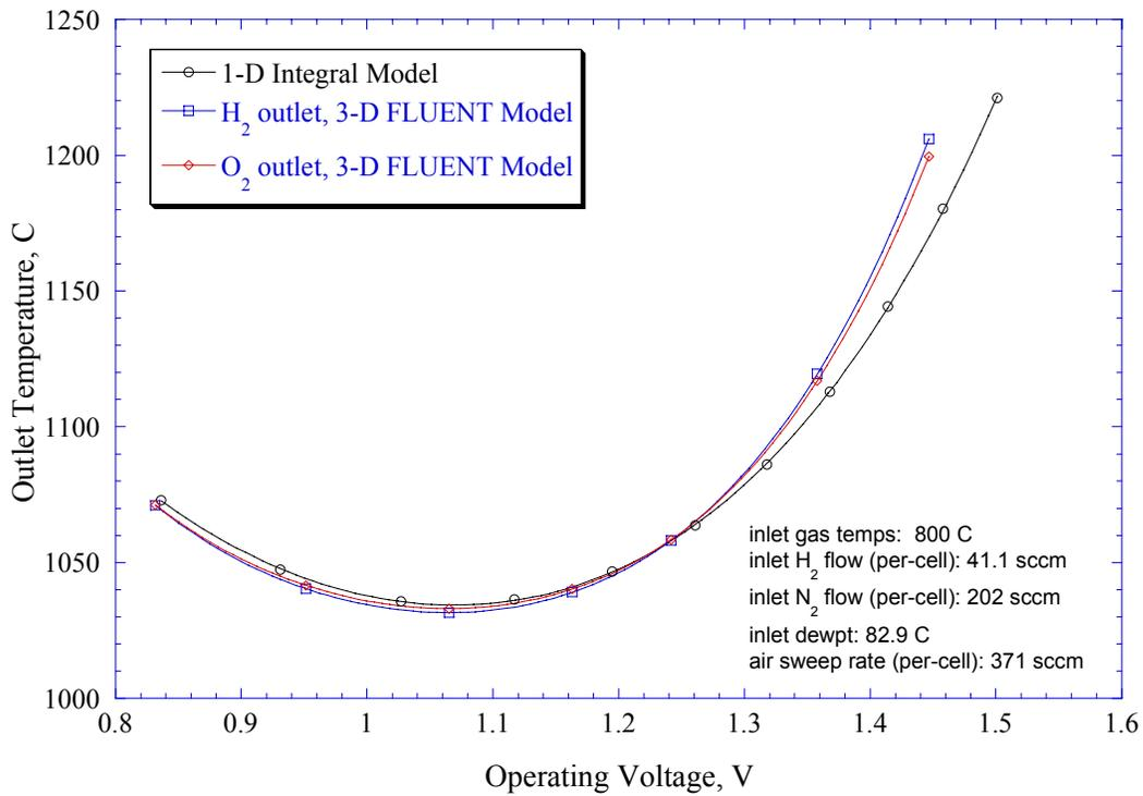
Figure 2. Predicted gas outlet temperatures for adiabatic electrolyzer operation; comparison of 1-D integral MathCad model with full 3-D FLUENT simulation.
