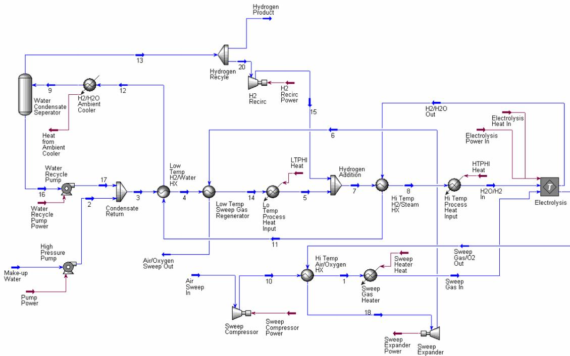
Figure 3. HYSYS process flow diagram for a 300 MW HTE plant with air sweep.
