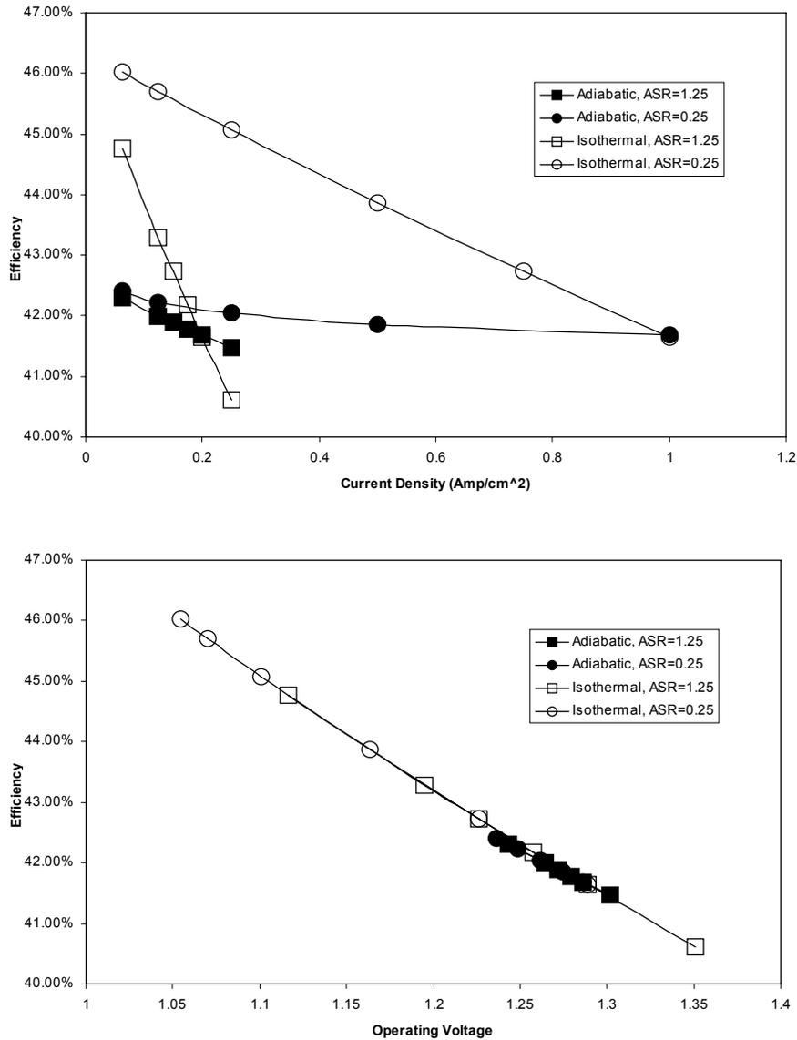
Figure 9. Overall thermal-to-hydrogen efficiencies (LHV) for Cases 9 – 12 (no sweep, fixed steam utilization, 1100 K electrolyzer inlet temperature, 5 MPa).
