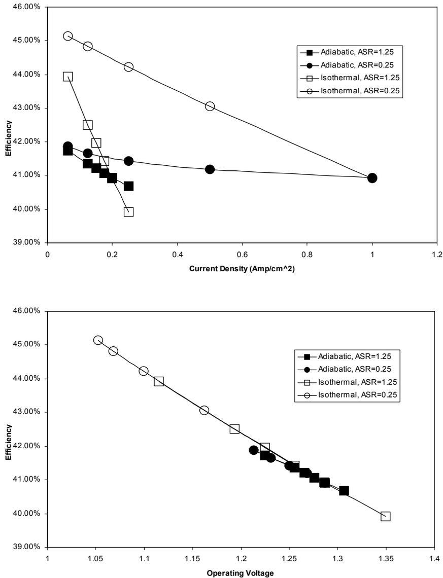
Figure 7. Overall thermal-to-hydrogen efficiencies (LHV) for Cases 1 – 4 (air sweep, fixed steam utilization, 1100 K electrolyzer inlet temperature, 5 MPa).
