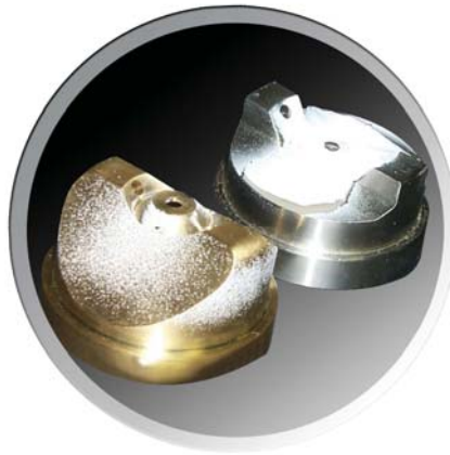
Figure 9 — 113AB air cap (forward, left) and 113 air cap (back, right) after 60 min. laboratory trial.
