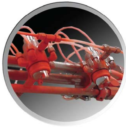
Fig. 10 — VAU-SS+113AB showing greatly reduced bearding after 1 hour during clinical trial.
