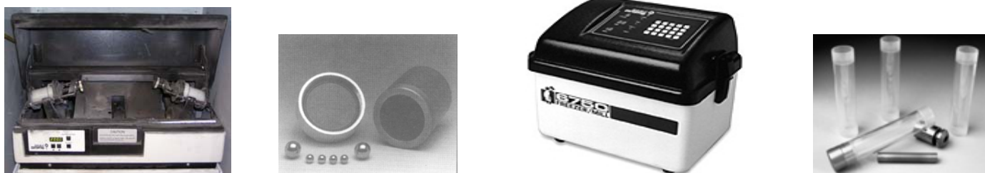
Figure 2 SPEX 8000 miller and stainless steel vials/media; SPEX 6750 cryogenic miller and polycarbonate vials with steel impactor.
