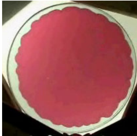
Figure 3. An image of the suspension/air interface rendered unstable by viscous miscible fingering. A 40% suspension of 100 \mu\text{m} glass spheres in glycerin was used in the experiment
