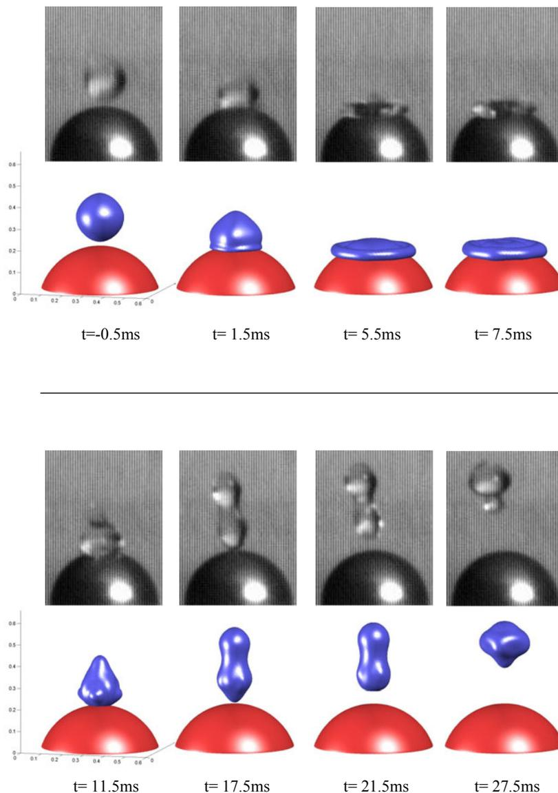
**Figure 3.** Experimental photos and simulated images of the 2.1mm acetone droplet impact on the 5.5mm particle at 250°C. The impact velocity is 45 cm/s. The unit for the coordinate is cm
