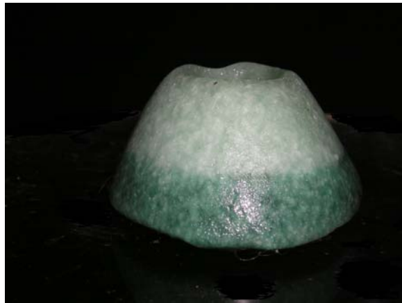
Figure 6. Photograph of a molten solid for a temperature of 30.8°C and after 254.1gms have melted. Base diameter = 4.9cm, Top diameter = 1.9cm and Height = 2.7cm.
