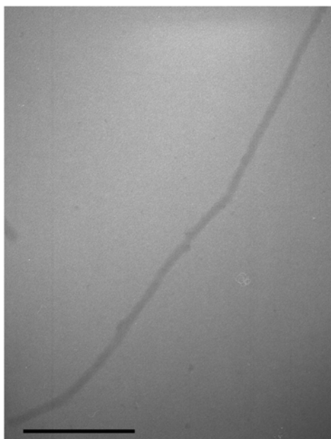
Figure 1: TEM image, unstained, of silica-coated wild-type TMV suspended in 100% MeOH. The scale bar is 200 nm.
