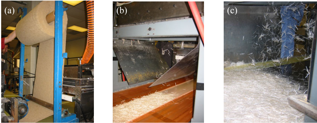
Figure 4. Continuous SMC compounding line utilizing: (a) non-woven hemp mat; (b) chopped hemp twine; and (c) hybrid mixture of chopped hemp twine and glass.
