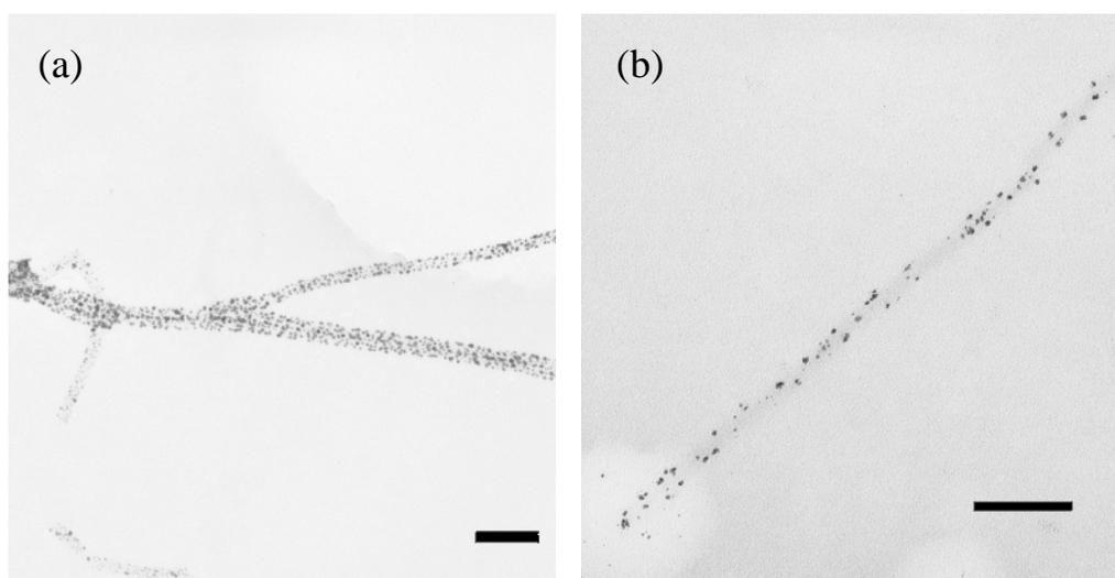
**Figure 2.** Platinum nanoparticle-deposited engineered TMV (a: Pt-deposited 2cysTMV. b: Pt-deposited E50Q. Scale bar: 100nm)
