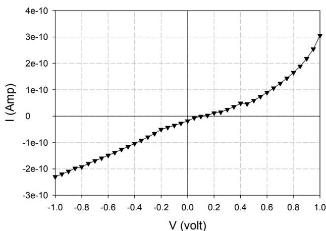
**Figure 3.** I-V curve of platinum-deposited 2cysTMV
