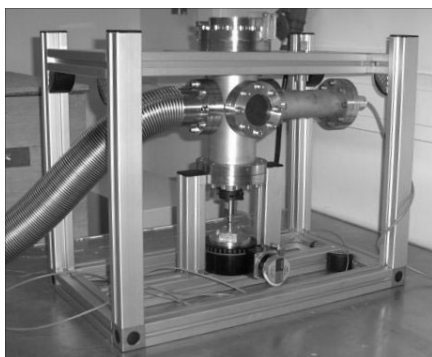
Figure 2: Picture of environmental vacuum chamber
