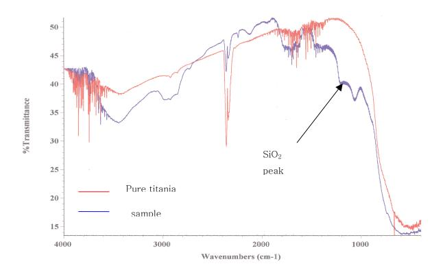
Figure 2. FTIR spectra of pure titania and modified titania particles
