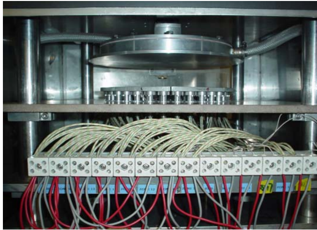
Figure 5: A programmable multizone thermal processing system.
